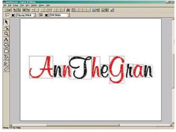
If you're setting up a phrase of more than one line of text, have the second line stitch from right to left, the third line from left to right and so on. This will avoid that long jump thread between rows. A long jump thread can catch the foot of your machine and throw the design out of registration or become buried in the next row of stitches and be difficult or impossible to trim neatly
